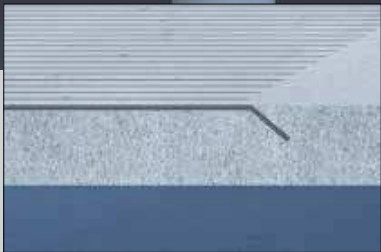
SikaWrap® FX for anchorage of near surface mounted (NSM) cantilevered applications
