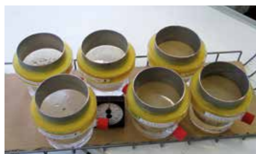
Water vapour transmission test
