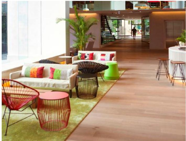
Adhering to the existing concrete, tile and ply subfloors, American Oak floor boards were fixed utilising SikaBond® - T55(J). Facilitating the speedy application, the easy flowing one-part polyurethane adhesive is designed for direct elastic bonding of timber floors. The adhesive is of low viscosity and cures on exposure to atmospheric moisture.
