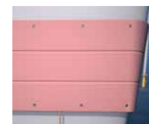
Curing by heater blanket for at least one hour at 80°C.
