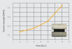
After 8 hours the final strength is reached (0.75 MPa). When the joints can be released strongly depends on the exposure they are omitted to. This can be after 1-2 hours for recessed floor joints or 4 hours for level joints with light pedestrian traffic. For further product data refer to technical data sheet.
