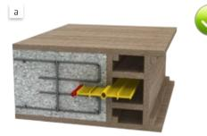
Fig. 5.101: Waterbar stop end formwork to the base slab
