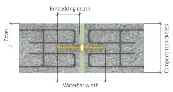
Fig. 5.17: "Width rule" for waterbars (width ≤ component thickness)
