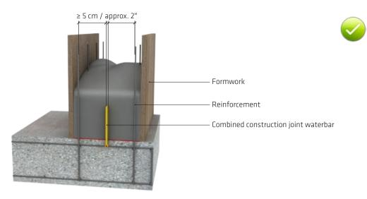
Fig. 7.13: Recommended clearance between Sika® KAB 125 or Sika® KAB 150 and the reinforcement
