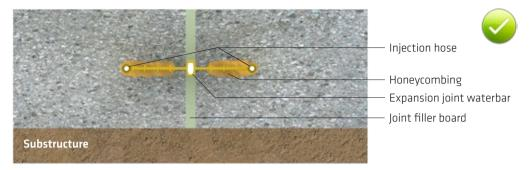
Fig. 15.9: Grouting of honeycombing and voids around the sealing part of the internal expansion joint waterbar through the installed injection hoses
