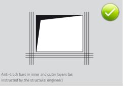
Fig. 2.9: Additional reinforcement at re-entrant corners of window openings to prevent diagonal cracking
