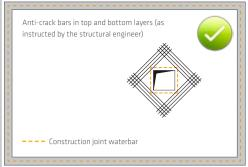
Fig. 2.7: Crack reduction bars at box-out and shafts to prevent diagonal cracking
