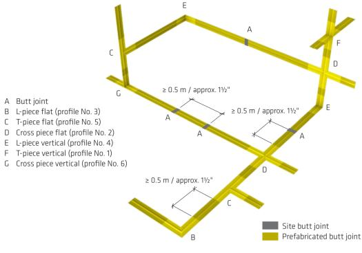
Fig. 5.64: Minimum spacing for prefabricated and site joint layout
