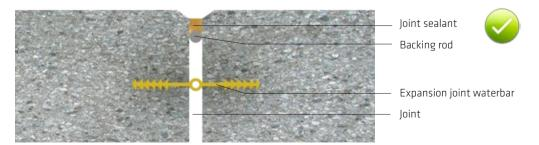
Fig. 14.8: Joint waterproofing with a Westec<sup>®</sup> internal expansion joint waterbar (type 050) and sealing with a suitable joint sealant (i.e. Sikaflex)
