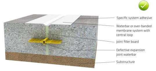
Fig. 15.13: Sealing of a leaking expansion joint with an over-banding membrane system
