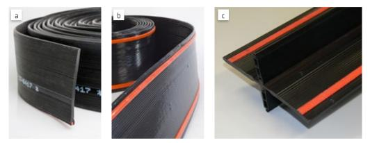
Fig. 7.2: Combined construction joint waterbars: Sika® KAB 125 or Sika® KAB 150 for horizontal construction joints between base slab and wall (a), Sika® KAB 175 S for vertical construction joints in walls (b), and Sika® KAB 175 SR for induced crack sections (c)
