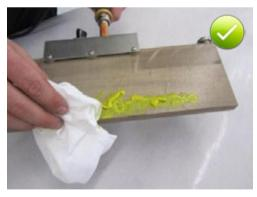
Fig. 5.70: Cleaning with a cloth to remove any welding residues from the welding blade before each welding operation
