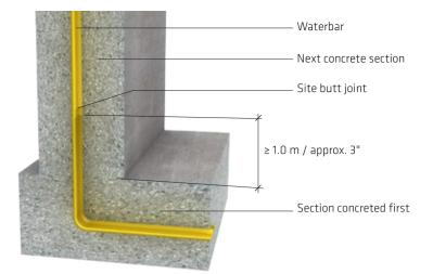
Fig. 5.34: Length of free connecting ends of a partially installed waterbar
