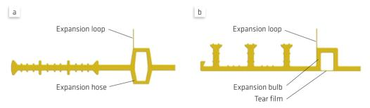
Fig. 5.94 Expansion bulb / hose (a) and tear flap closed expansion loop (b) on Sika PVC-P waterbars with their nail strap
