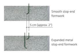
Fig. 9.18: Sample installation drawing with the associated standard details [8]
