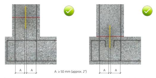
Fig. 5.27: Minimum clearance between an internal construction joint waterbar and the starter bars, using the example of a base slab-wall joint with a concrete kicker (left) and top reinforcement break (right)
