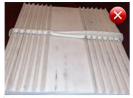
a Weld does not cover the full waterbar width/thickness
