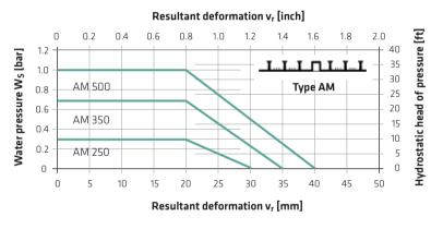
Fig. 5.53: Selection diagram for external elastomeric expansion joint waterbars (type: AM) according to DIN 18197 [7]
