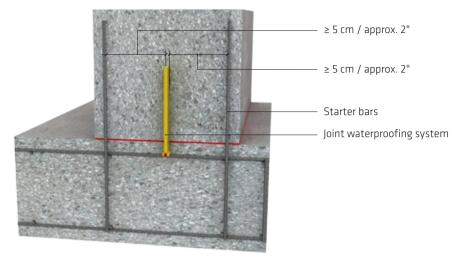
Fig. 3.7: Recommended minimum clearance between joint waterbars and steel starter bar
