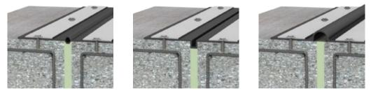
Fig. 5.14: Flanged waterbars with legs (flanges) clamped on both sides of the joint
