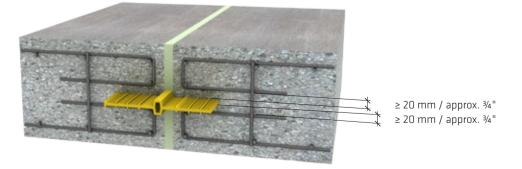
Fig. 3.6: Recommended minimum clearance between the reinforcement and joint waterbars
