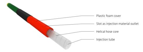
Fig. 9.8: Structure of the SikaFuko® Eco-1 injection hose
