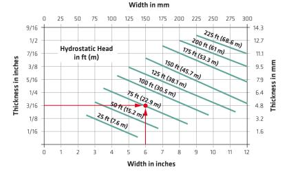
Fig. 5.40: Determination of the permissible water pressure (Hydrostatic Head) for an expansion joint waterbar (width: 6" / 152 mm, thickness: 3/16") from US Army Corps of Engineers "Waterstops and other joint materials" (EM1110-2-2102)
