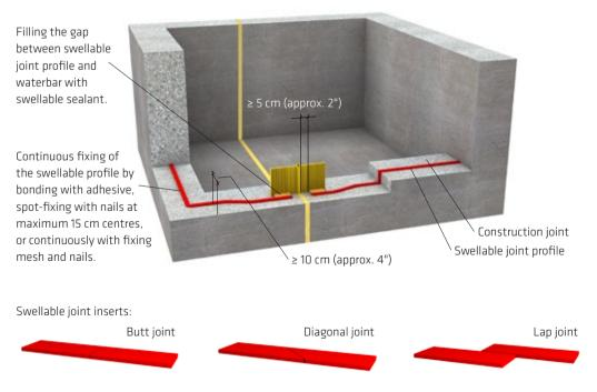
Fig. 8.9: Minimum clearances and how to install SikaSwell® swellable profiles
