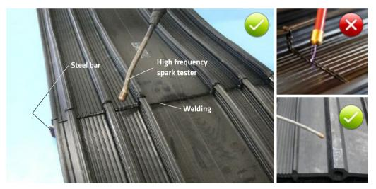
Fig. 5.85: Non-destructive testing of the impermeability of a weld with a high frequency spark tester; a visible spark passing through indicates a defect in the weld
