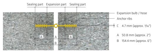
Fig. 14.4: Westec® internal expansion joint waterbar (type 050) complying with European Technical Approval ETA 04/0044 for LAU installations [7]
