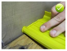
Fig. 5.69: Melting process at the waterbar end in contact with the hot welding blade  $% \left( {{{\rm{D}}_{\rm{B}}}} \right)$
