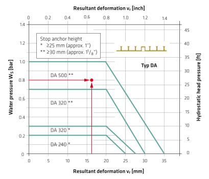
Fig. 5.45: Selection of a Sika® Tricosal® Tricomer® external expansion joint waterbar (example 1)
