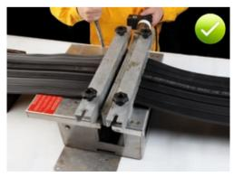
Fig. 5.74: Fusing the waterbar ends together by pressing them onto the hot welding blade with the closing lever mechanism
