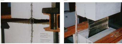
Fig. 5.49: Tensile test on a Sika® Tricosal® Tricomer® internal expansion joint waterbar 32 cm (approx. 121/2") in width
