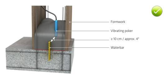
Fig. 7.14: Minimum clearance between KAB profile and vibrating pokers
