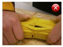
Fig. 5.83: Breaking the weld open in the cold bending test on an incorrectly welded butt joint
