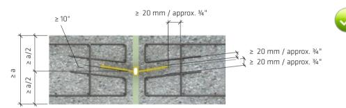
Fig. 5.30: V-shaped installation of internal waterbars in horizon¬tal and slightly inclined components (a: waterbar width)
