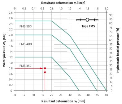
Fig. 5.55: Selection of a Sika® Tricosal® internal elastomeric expansion joint waterbar (type FMS)
