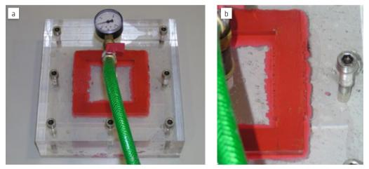
Fig. 8.7: Swelling test on SikaSwell<sup>®</sup> A, in which the swellable tape has expanded into the micro-gap between the two test plates and sealed it (a: test assembly, b: detail of the swellable profile expanded into the available micro-gap)
