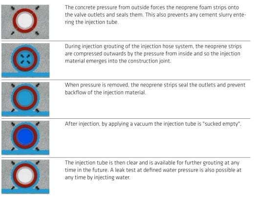
Fig. 9.9: How the SikaFuko® Eco-1 injection hose works
