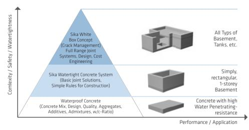
Fig. 2.1: Overview of Sika Waterproof Concrete, Sika Watertight Concrete Systems and the Sika White Box Concept
