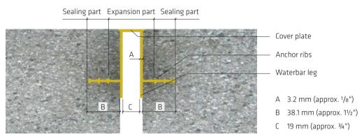
Fig. 14.3: Westec® end waterbar (type 631) complying with European Technical Approval ETA 04/0044 for LAU facilities [7]
