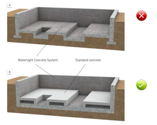
Fig. 2.4: Examples of unsuitable (a) and suitable (b) basement design configurations for selection of a Sika Watertight Concrete System
