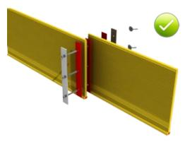
Fig. 7.9: Butt joint in a Sika $^{\circ}$  KAB 150 with clamping bars and swellable profile insert
