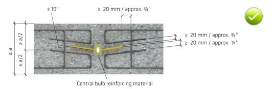
Fig. 5.32: Waterproofing of a connection joint in which shear strain occurs using an expansion joint waterbar with a reinforced central bulb (a = waterbar width)
