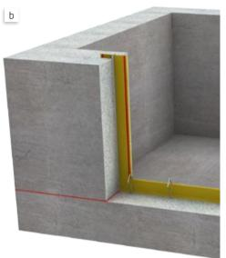
Fig. 4.3: Crack inducers for forming controlled crack induced joints (a: controlled crack sealing tube, b: KAB 175 SR)
