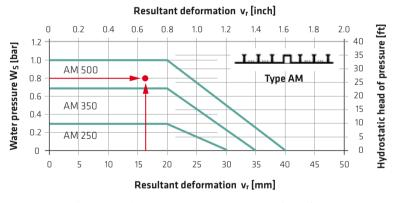
Fig. 5.56: Selection of a Sika® Tricosal® external elastomer expansion joint waterbar (type AM)
