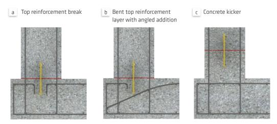
Fig. 5.20: Waterproofing of base slab-wall construction joint with an internal waterbar
