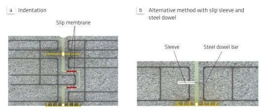
Fig. 5.33: Waterproofing of an expansion joint with transverse force transmission
