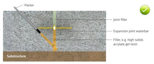
Fig. 15.10: Injection sealing of a joint with a damaged expansion part of the waterbar
