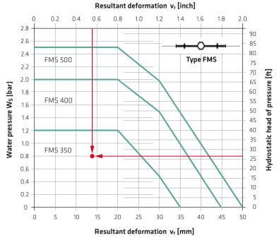
Fig. 5.58: Selection of a Sika® Tricosal® internal elastomer expansion joint waterbar (type FMS)
