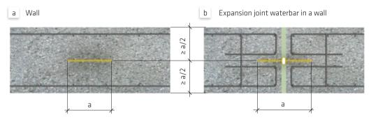
Fig. 5.19: Examples of correct waterbar configuration
