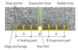
Fig. 5.10: Geometry and functions of different expansion joint waterbar profiles
