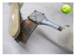
Fig. 5.79: Removing residues from the heating surfaces of a welding axe with a wire brush before the next welding operation
