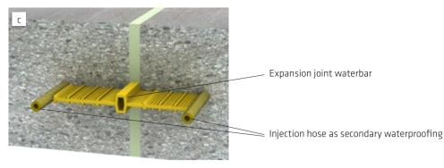
Fig. 9.3: Injection hose systems for primary (a) and secondary waterproofing (b, c)
