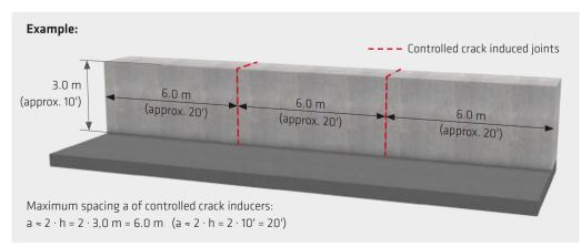
Fig. 3.4: Sample calculation for the spacing of controlled crack induced joints in a wall
