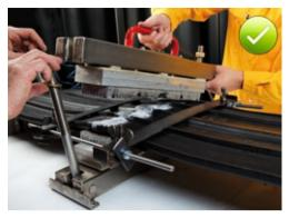
Fig. 5.87: Tensioning the vulcanizer
