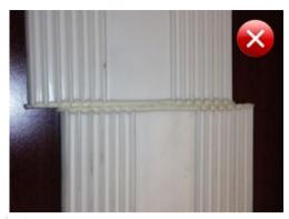
b The waterbar profiles out of line in the welded joint
