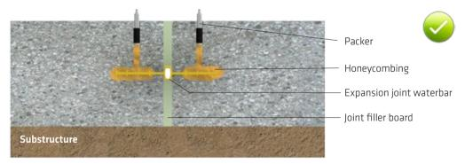
Fig. 15.8: Grouting of voids around the sealing part of an internal expansion joint waterbar
