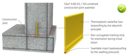
Fig. 7.1: Structure and installation positioning of Sika® KAB 125 / Sika® KAB 150
