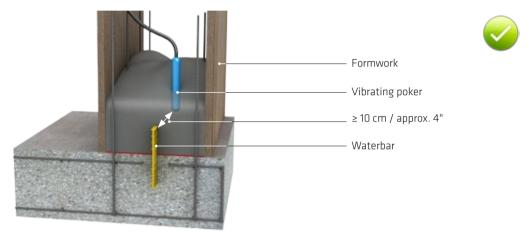
Fig. 5.104: Minimum clearance to the waterbar and other joint sealing parts of waterstop systems for compacting the concrete with a vibrating poker
