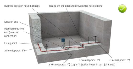
Fig. 9.14: Minimum clearances recommended for the installation of injection hose systems
