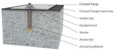
Fig. 13.3: Typical schematic layout of a clamped flange joint seal
