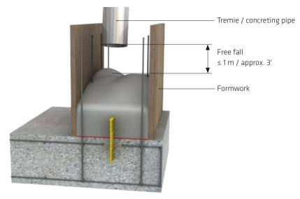
Fig. 2.20: Recommended maximum free fall when concreting walls
