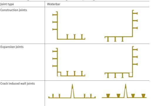
All waterbars tend to have characteristic profile and geometry. Figs. 5.10 – 5.12 illustrate this with the profiles of different expansion and construction joint waterproofing products, generally the waterbars will comprise a sealing part and where required, an expansion / deformation part.
