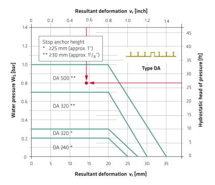
Fig. 5.47: Selection of a Sika® Tricosal® Tricomer® external construction joint waterbar (example 2)
