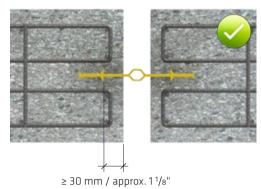
Fig. 5.95: Anchorage of internal expansion joint waterbar with  $\ge$  30mm
