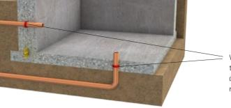
Waterproof sealing around pipe penetrations and conduits etc., e.g. sealing collars, swellable profiles or annular ring seal gaskets
