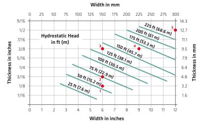
Fig. 5.41: Permissible water pressure for the sample waterstops in Table 5.16 according to Corps of Engineers "Waterstops and other joint materials" (EM1110-2-2102), Nos. 1 – 5 refer to the waterbars in Table 5.16.
