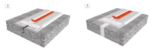
Fig. 10.2: Schematic diagram of the joint sealing solution for a crack (a) and a construction joint (b) with Sikadur-Combiflex® SG
