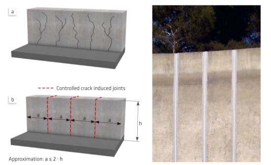
Fig. 3.3: Arrangement of controlled crack induced joints (a: random cracking in wall without joints, b: wall with crack induced joints)
