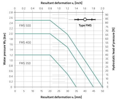
Fig. 5.52: Selection diagram for internal elastomer expansion joint waterbars with lateral steel straps (type: FMS) according to DIN 18197 [7]
