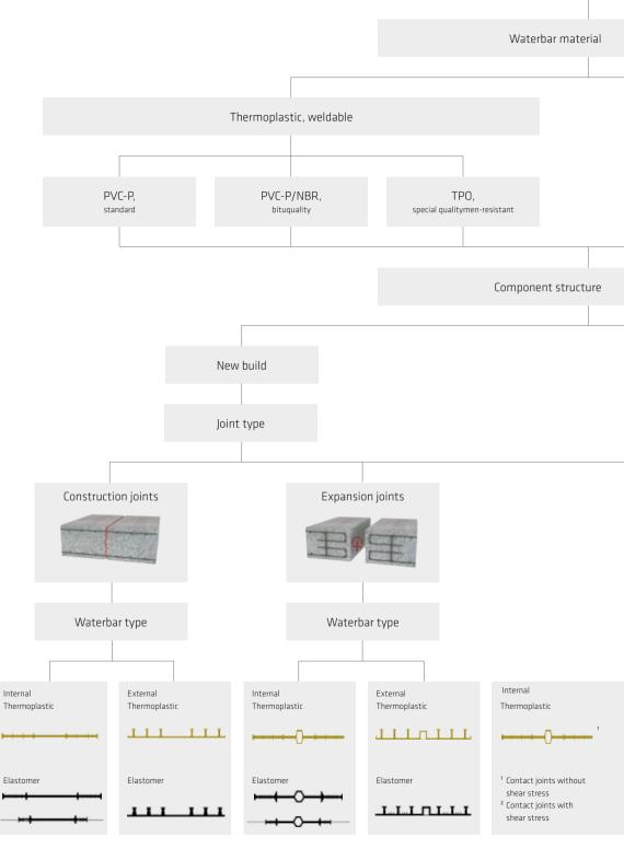
Fig. 5.4: An overview of different waterbars and their uses
