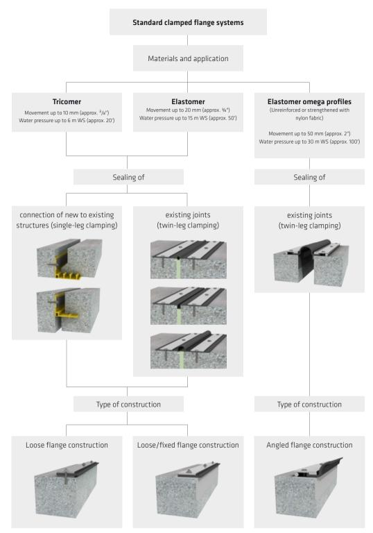
Fig. 13.2: Different clamped flange expansion joint sealing system designs
