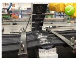
Fig. 5.89: Butt joint after vulcanisation
