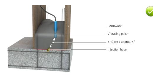
Fig. 9.17: Minimum clearances between injection hose and vibrating poker
