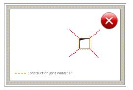
Fig. 2.6: Diagonal cracks at box-outs or shafts through a base slab
