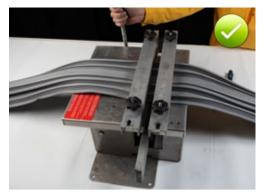
Fig. 5.75: Pressing the molten waterbar ends together with the closing lever mechanism again after lowering the blade
