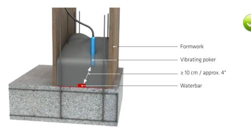
Fig. 8.10: Minimum clearances between swellable profile and vibrating poke
