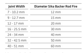
Joints need to be deep enough to accomodate appropriate size Sika Backer Rod Fire, plus sealant depth.
