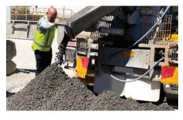
Unload the granulated materials after the treatment in a covered area in layers, no more than 25 cm thick;
