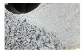
Mix at maximum speed, 1 minute/treated cubic metre or till the concrete granulates;
