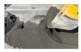
Rework quickly (lift-remix) the granulated by-product by using the wheel loader in use at the batching plant after 3-4 hours from the initial process. Keep the material in dry conditions for at least 24 hours.
