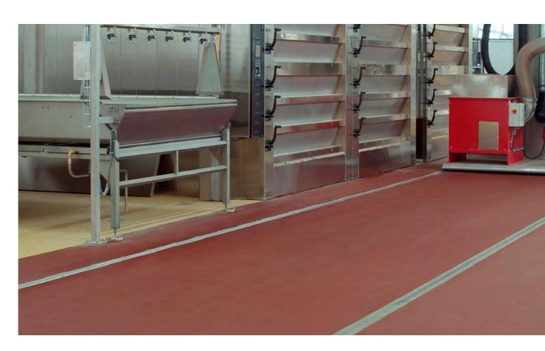
As to the floor area in immediate vicinity of the large ovens additional features were required: due to the strong heat during the baking process, an extremely heat tolerant, hygienic flooring system is required. Proven to be ideal for this, Sikafloor® PurCem® HS-21 with high chemical, mechanical and thermal resistance was applied. It is a heavy-duty resistant, multifunctional floor system that has years of proven records for use in sensitive areas such as production of the food industry.
