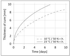
Diagram 1: Curing speed Sikaflex®-527 AT
