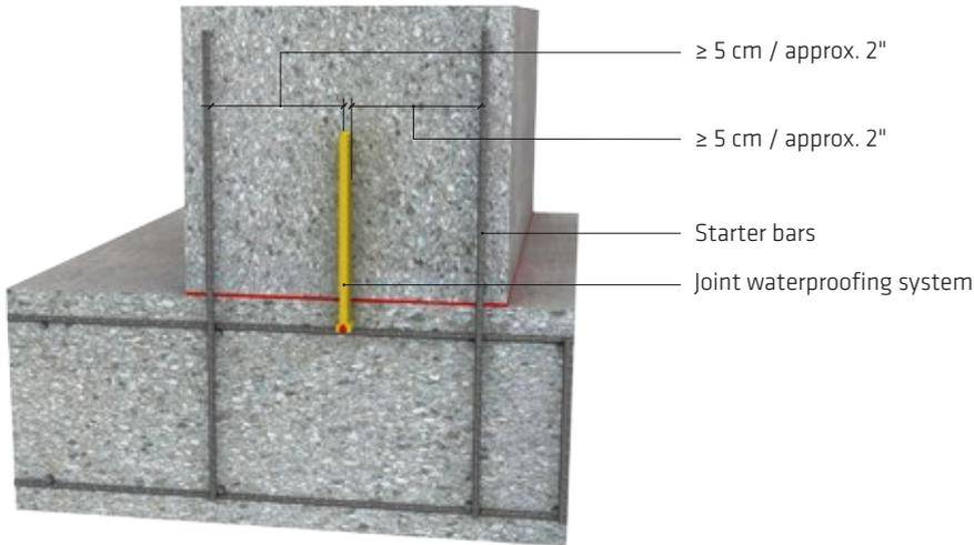
Fig. 3.7: Recommended minimum clearance between joint waterbars and steel starter bar
