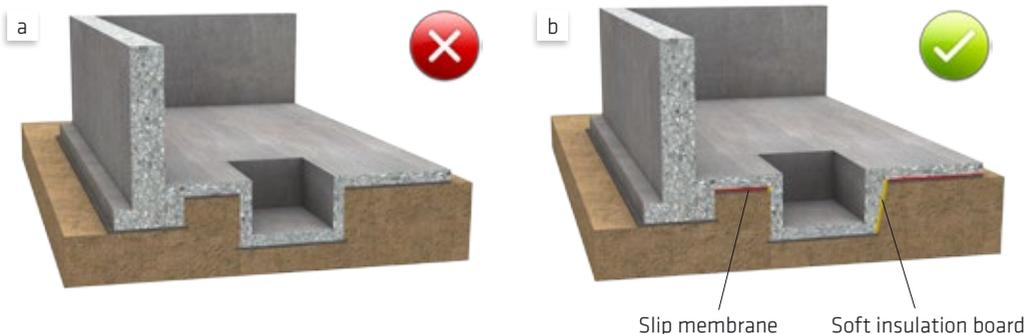
Fig. 2.16: Design of additional features in the base slab, e.g. for a lift pit (Example a): unsuitable, (Example b): suitable
