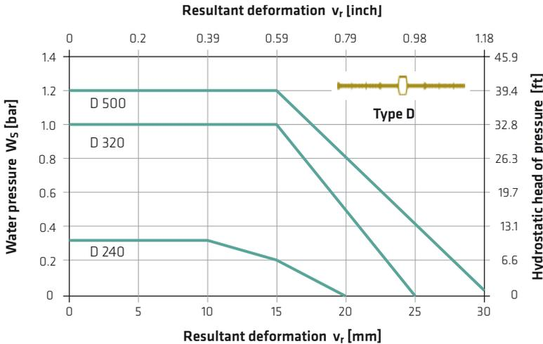
Fig. 5.43: Selection diagram for Sika® Tricosal® Tricomer® internal expansion joint waterbars according to DIN 18197 [7]
