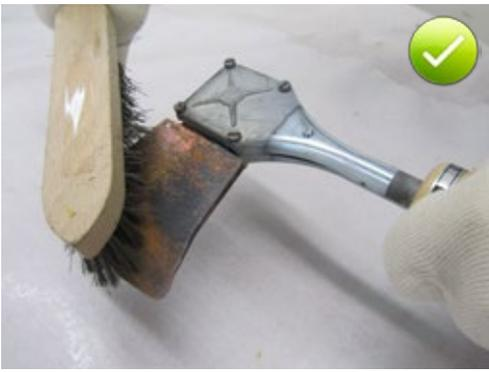
Fig. 5.79: Removing residues from the heating surfaces of a welding axe with a wire brush before the next welding operation
