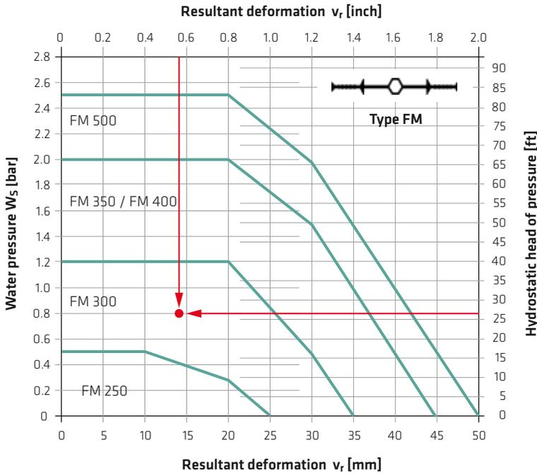
Fig. 5.57: Selection of a Sika® Tricosal® internal elastomer expansion joint waterbar (type FM)
