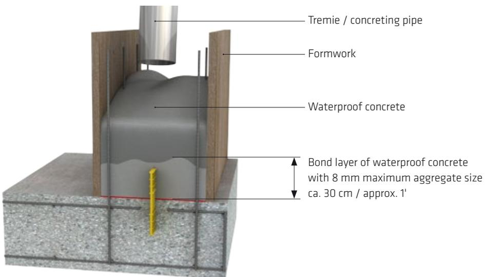
Fig. 2.21: Bond layer mix with a maximum aggregate diameter of 8 mm (approx. 1') that is usually recommended when concreting walls
