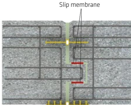
b Alternative method with slip sleeve and steel dowel
