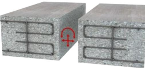
Movement or expansion joints split components through their full thickness with a joint gap of defined width. The reinforcement in movement joints is discontinuous. Movement / expansion joints allow differential movement due to temperature variations and / or load / settlement in one or more directions of the areas, sections or structures separated by the joint.
