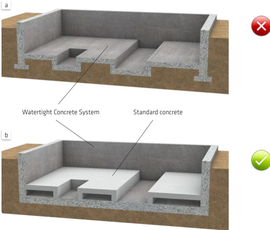
Fig. 2.4: Examples of unsuitable (a) and suitable (b) basement design configurations for selection of a Sika Watertight Concrete System
