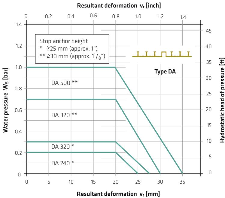
Fig. 5.44: Selection diagram for Sika® Tricosal® Tricomer® external expansion joint waterbar according to DIN 18197 [7]
