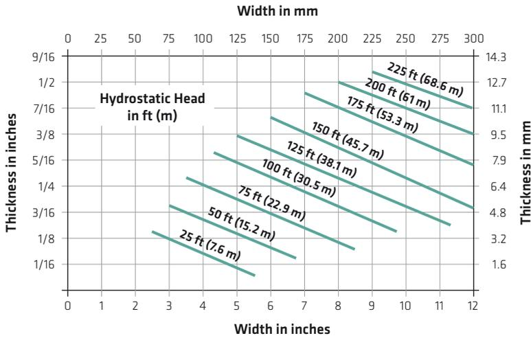
Fig. 5.39: Water pressure dependent dimensions of waterbars according to the US Army Corps of Engineers “Waterstops and other joint materials” (EM1110-2-2102)
