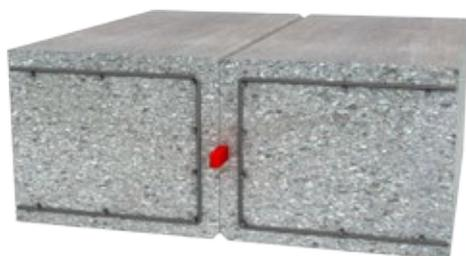
Waterproofing of a connection joint with dimensionally stable swelling profile, e.g. SikaSwell®-P (if no joint opening is expected)
