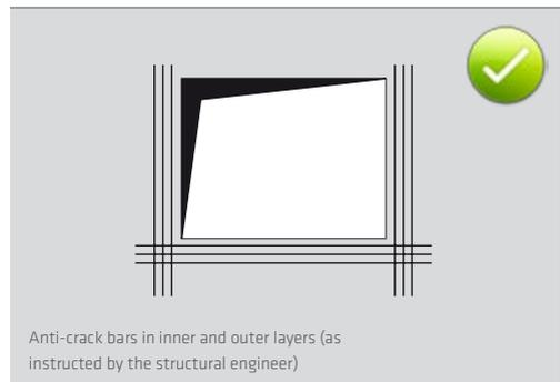
Fig. 2.9: Additional reinforcement at re-entrant corners of window openings to prevent diagonal cracking
