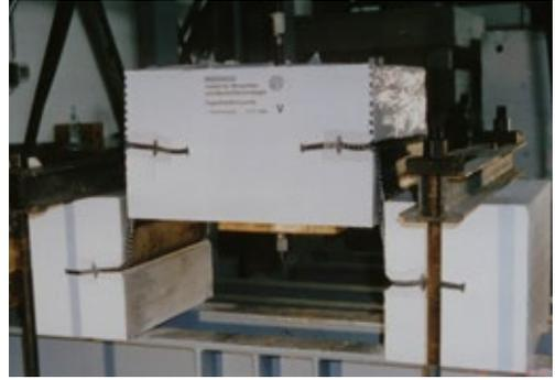
Fig. 5.50: Shear test on a Sika® Tricosal® Tricomer® internal expansion joint waterbar 32 cm (approx. 12½") in width
