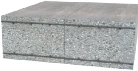
Construction joints are designed to split areas of the structure into separate concrete sections for work scheduling reasons, or as a structural measure to transfer load for example. The reinforcement in construction joints is therefore continuous through the joint.
