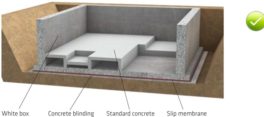
Fig. 2.15: An appropriate design for the Sika White Box Concept: a simple shape, uniform floor and wall thickness, no offsets
