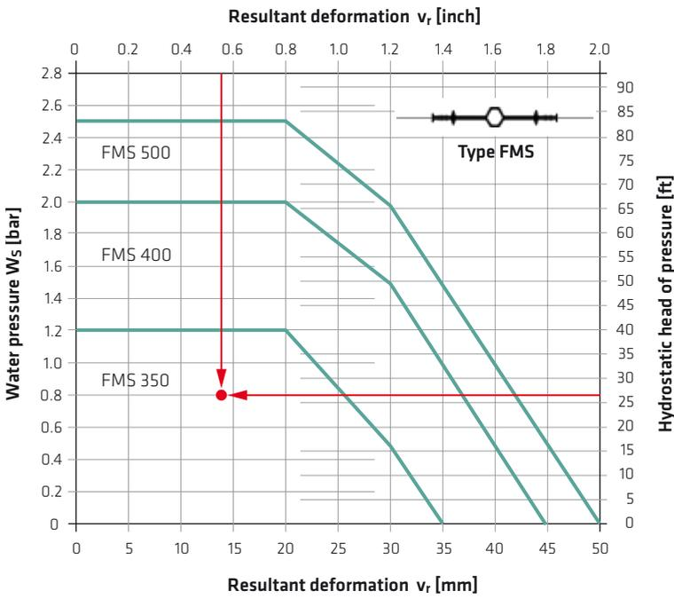
Fig. 5.58: Selection of a Sika® Tricosal® internal elastomer expansion joint waterbar (type FMS)
