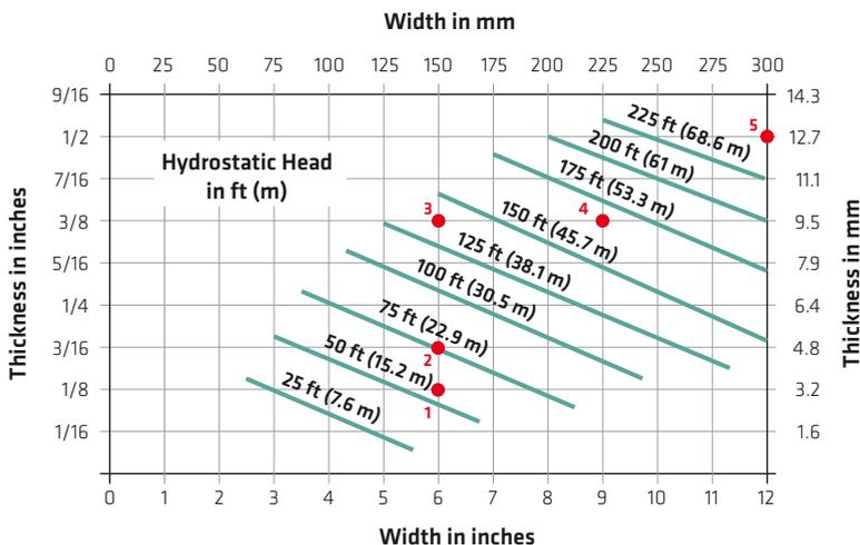
Fig. 5.41: Permissible water pressure for the sample waterstops in Table 5.16 according to Corps of Engineers "Waterstops and other joint materials" (EM1110-2-2102). Nos. 1 - 5 refer to the waterbars in Table 5.16.
