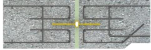
Fig. 5.18: Example of enlargement of a thin component to maintain the required thickness over the waterbar in its immediate area
