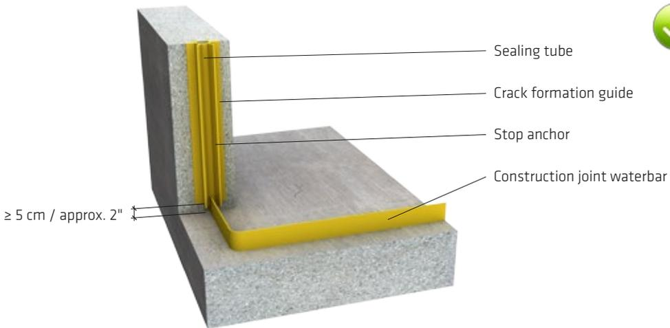
Fig. 11.5: Design of the base of the wall for installation of crack inducing sealing tubes
