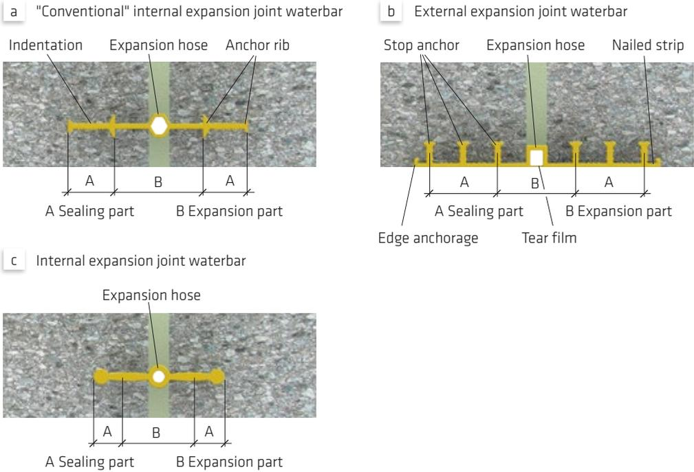
Fig. 5.10: Geometry and functions of different expansion joint waterbar profiles
