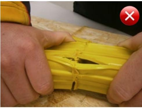
Fig. 5.83: Breaking the weld open in the cold bending test on an incorrectly welded butt joint
