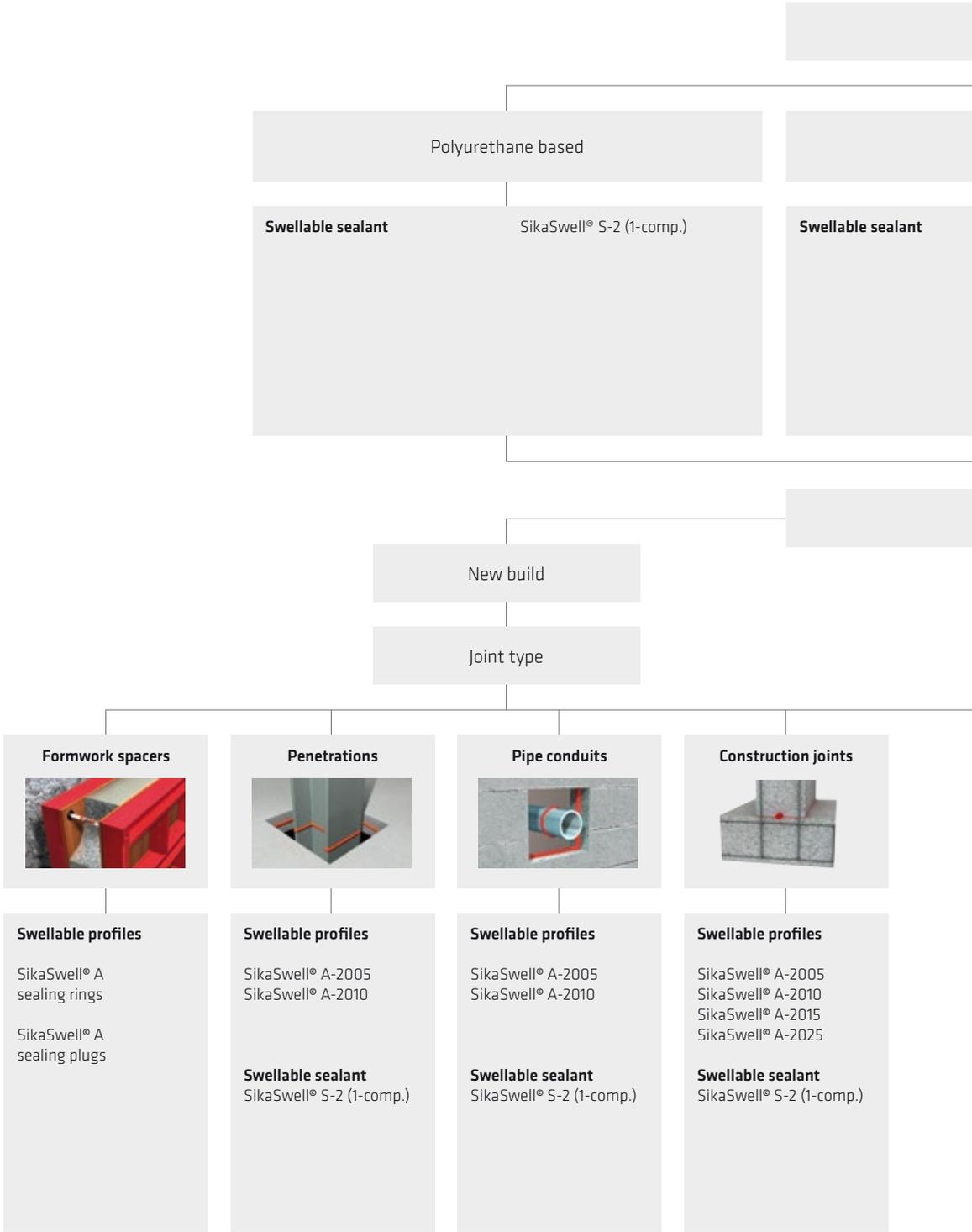
Fig. 8.3: Waterproofing with SikaSwell® - The different materials, forms and uses
