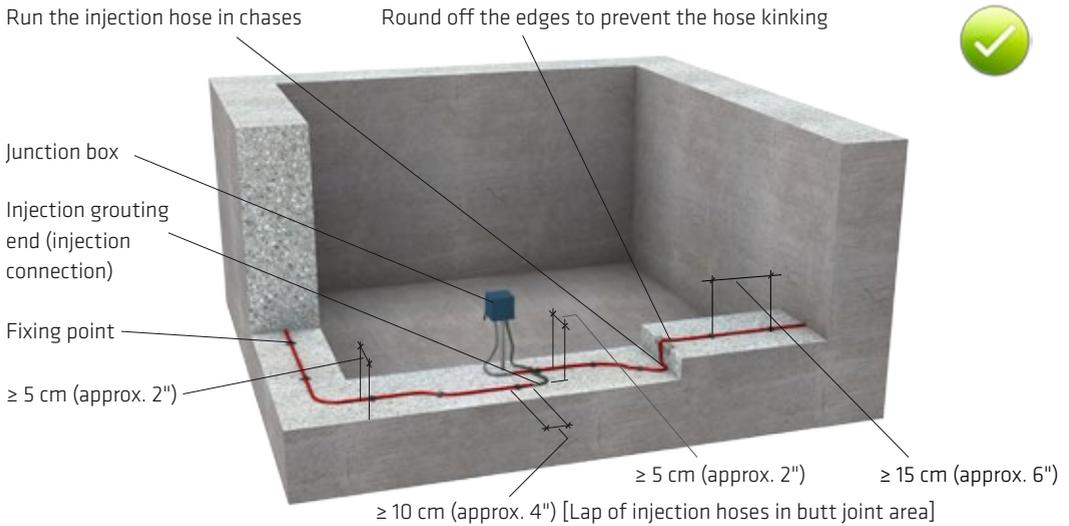
Fig. 9.14: Minimum clearances recommended for the installation of injection hose systems
