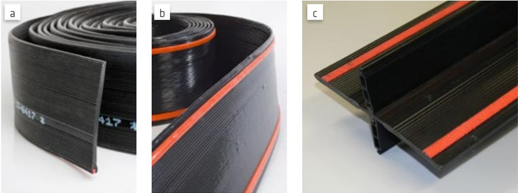
Fig. 7.2: Combined construction joint waterbars: Sika® KAB 125 or Sika® KAB 150 for horizontal construction joints between base slab and wall (a), Sika® KAB 175 S for vertical construction joints in walls (b), and Sika® KAB 175 SR for induced crack sections (c)
