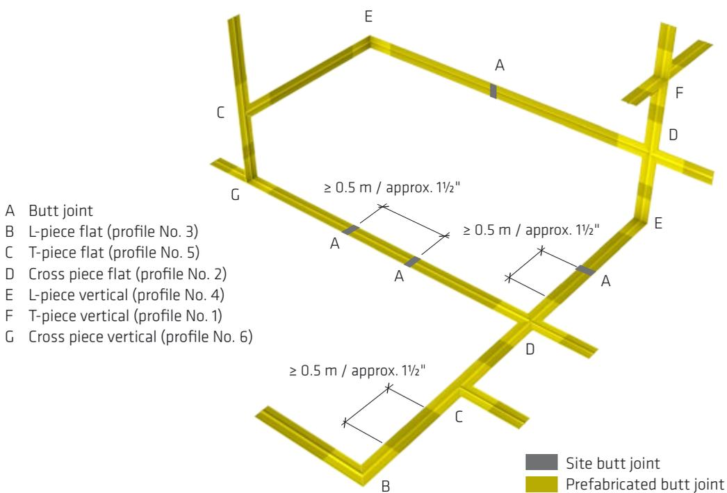
Fig. 5.64: Minimum spacing for prefabricated and site joint layout
