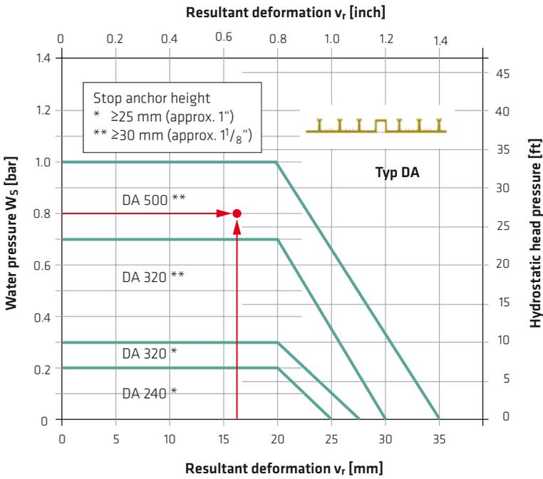
Fig. 5.45: Selection of a Sika Tricosal® Tricomer® external expansion joint waterbar (example 1)
