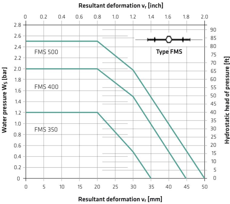
Fig. 5.52: Selection diagram for internal elastomer expansion joint waterbars with lateral steel straps (type: FMS) according to DIN 18197 [7]
