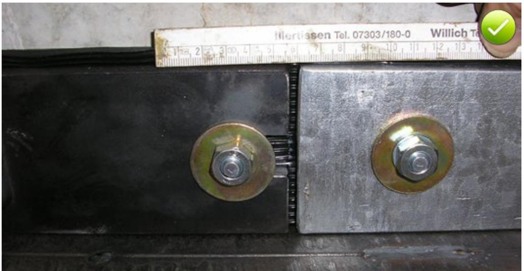
Fig. 13.6: Example of the correct spacing between two clamping flanges
