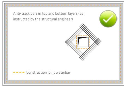
Fig. 2.7: Crack reduction bars at box-out and shafts to prevent diagonal cracking
