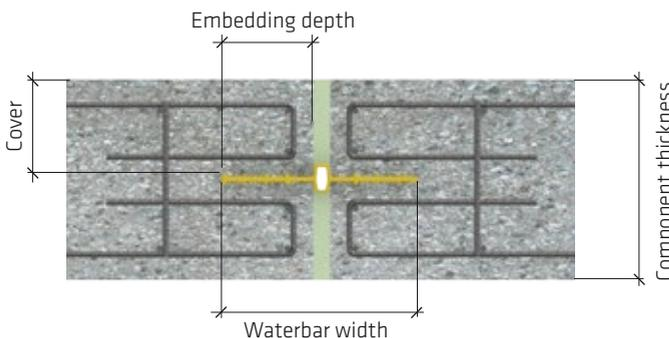
Fig. 5.17: "Width rule" for waterbars (width  $\leq$  component thickness)
