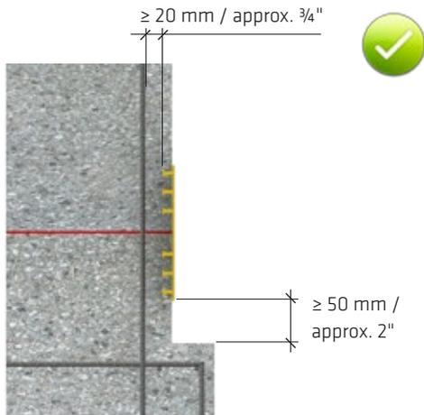
Fig. 5.23: Waterproofing of base slab wall-construction joint with an external waterbar
