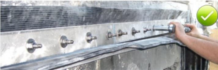
Fig. 13.8: Retightening the clamp to the specified tightening torque
