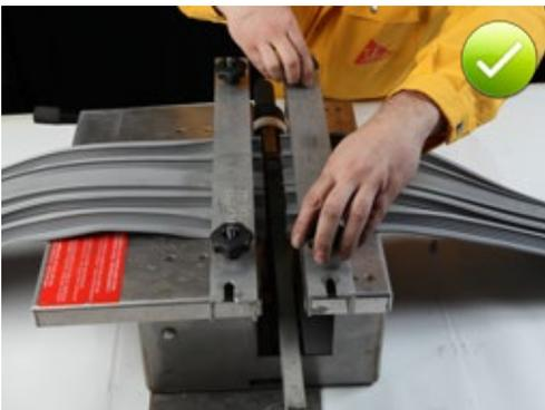
Fig. 5.73: Clamping the two waterbar ends in the SG 320 L automatic welding machine
