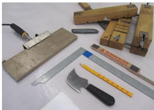
Fig. 5.65: Tools for heat welding of thermoplastic waterbars with a simple welding jig for butt joints
