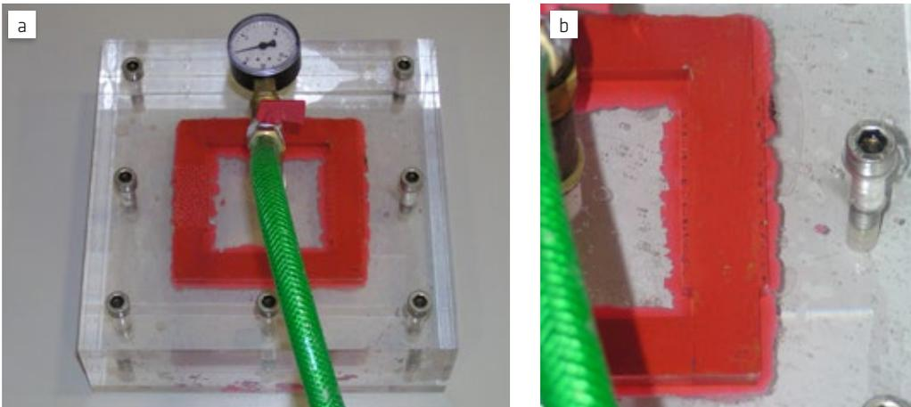
Fig. 8.7: Swelling test on SikaSwell® A, in which the swellable tape has expanded into the micro-gap between the two test plates and sealed it (a: test assembly, b: detail of the swellable profile expanded into the available micro-gap)
