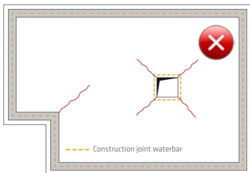
Fig. 2.17: Diagonal cracks in a base slab at re-entrant corners and box-outs etc.
