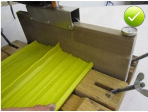
Fig. 5.66: Placing the waterbar ends in the jig and tightening the clamping bars
