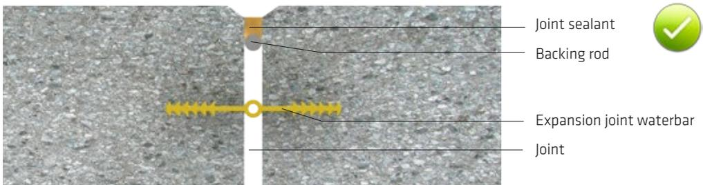
Fig. 14.8: Joint waterproofing with a Westec® internal expansion joint waterbar (type 050) and sealing with a suitable joint sealant (i.e. Sikaflex)
