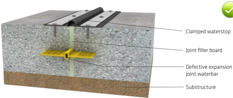
Fig. 15.11: Post-sealing of a leaking expansion joint with a clamped waterstop
