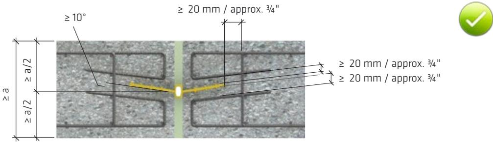
Fig. 5.30: V-shaped installation of internal waterbars in horizontal and slightly inclined components (a: waterbar width)
