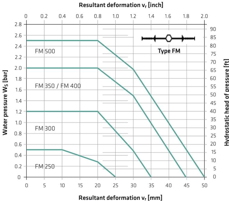
Fig. 5.51: Selection diagram for internal elastomer expansion joint waterbars (type: FM) according to DIN 18197 [7]
