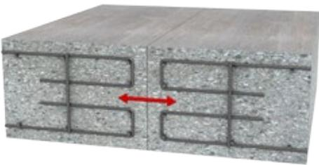
Connection joints are flat or indented joints which split the concrete section through its full thickness without a defined joint gap. The reinforcement in connection joints is discontinuous. When the concrete section contracts, joint movement (joint opening) is possible, and when it expands, pressure transmission is possible.
