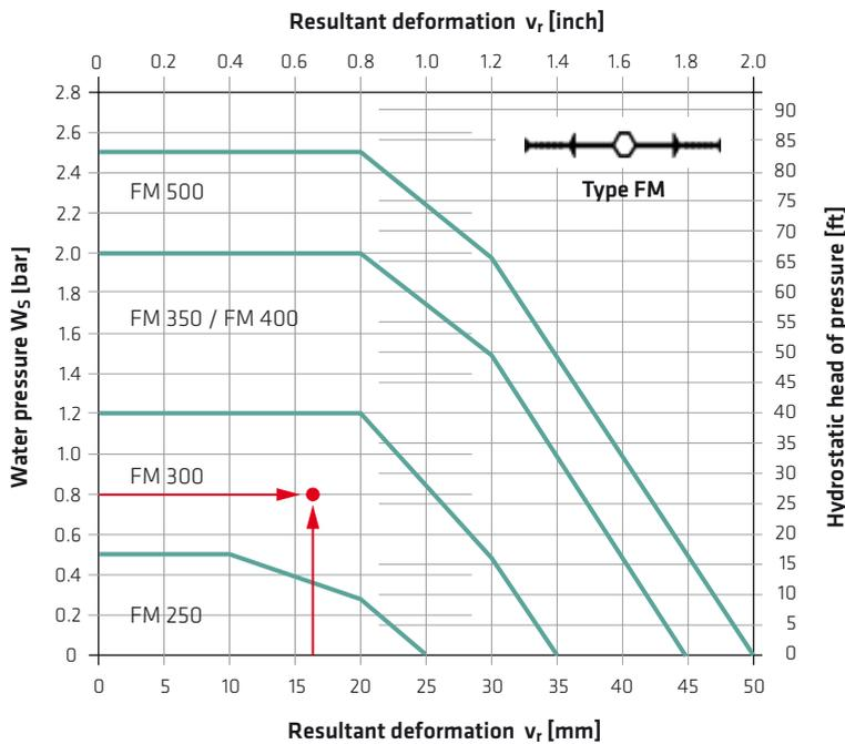
Fig. 5.54: Selection of a Sika® Tricosal® internal elastomer expansion joint waterbar (type FM)
