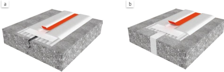
Fig. 10.2: Schematic diagram of the joint sealing solution for a crack (a) and a construction joint (b) with Sikadur-Combiflex® SG
