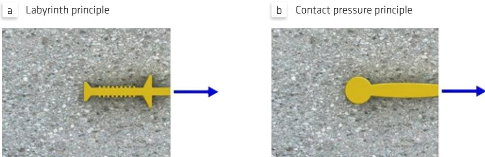
Fig. 5.11: Waterproofing principles of internal waterbars
