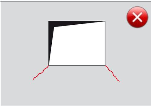
Fig. 2.8: Diagonal cracks at the corners of window openings
