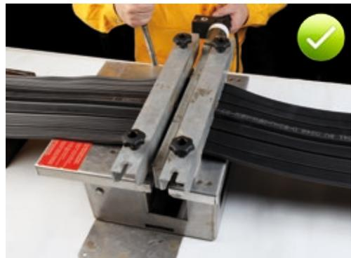
Fig. 5.74: Fusing the waterbar ends together by pressing them onto the hot welding blade with the closing lever mechanism
