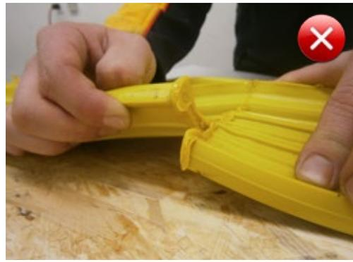
Fig. 5.84: Tearing the weld at an incorrectly welded butt joint
