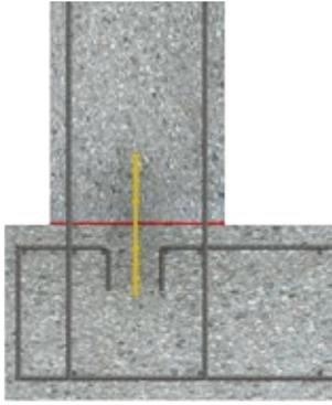
b Bent top reinforcement layer with angled addition
