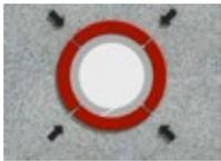
The concrete pressure from outside forces the neoprene foam strips onto the valve outlets and seals them. This also prevents any cement slurry entering the injection tube.
