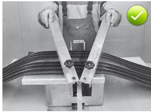
Fig. 5.76: Removing the finished butt joint from the SG 320 L automatic welding machine
