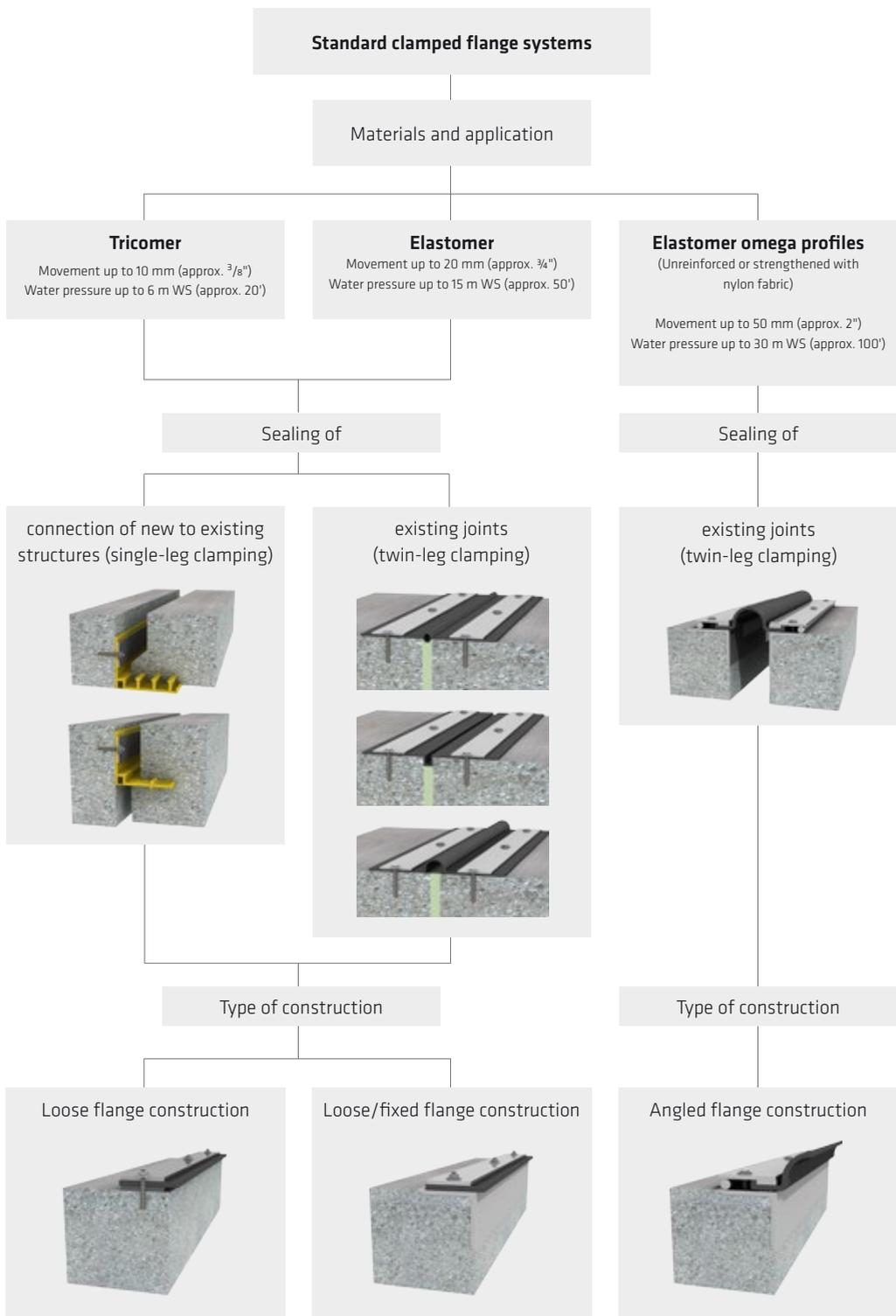
Fig. 13.2: Different clamped flange expansion joint sealing system designs
