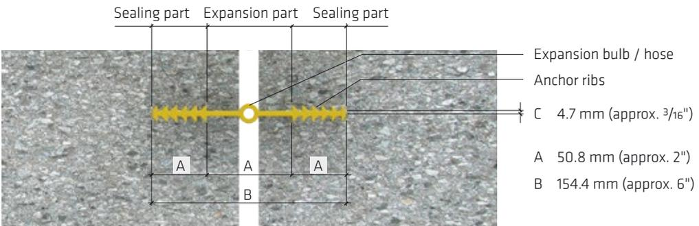
Fig. 14.4: Westec® internal expansion joint waterbar (type 050) complying with European Technical Approval ETA 04/0044 for LAU installations [7]
