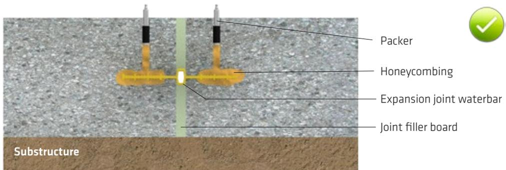
Fig. 15.8: Grouting of voids around the sealing part of an internal expansion joint waterbar
