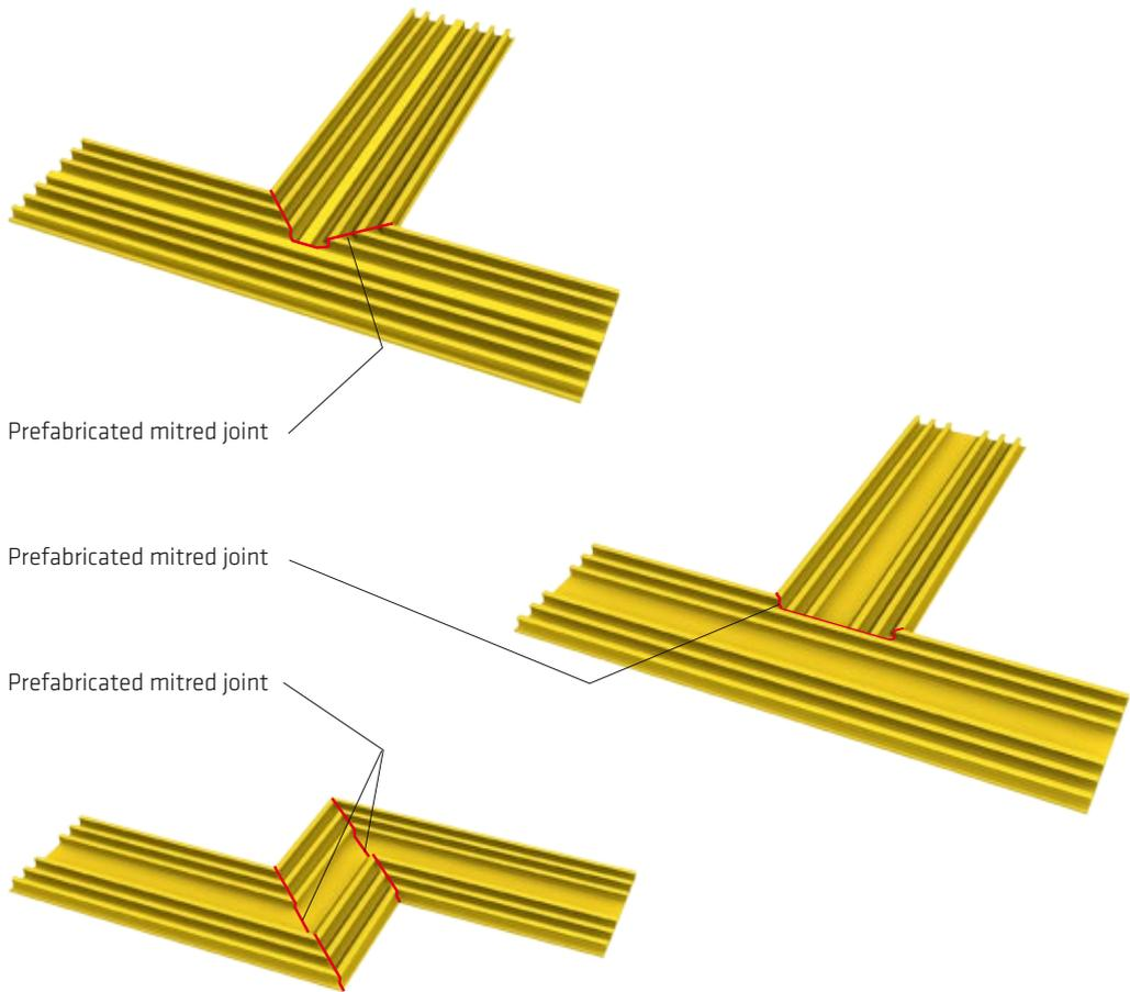
Fig. 5.63: Examples of correctly welded waterbar butt joints [8]
