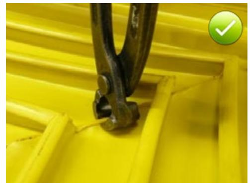
Fig. 5.71: Cutting to remove any excess areas or lengths of welding bead
