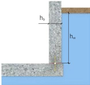
The example in Fig. 2.13 shows how to determine the maximum permitted crack width  $w_{cal}$  to utilise the self-healing approach for any cracks that do occur:
