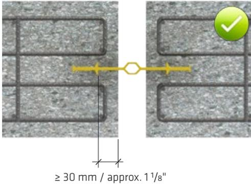
Fig. 5.95: Anchorage of internal expansion joint waterbar with  $\geq 30$  mm concrete cover
