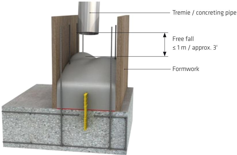
Fig. 2.20: Recommended maximum free fall when concreting walls
