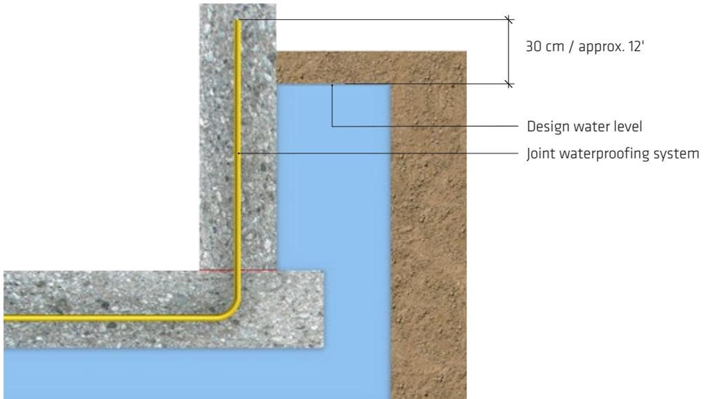
Fig. 3.5: Minimum height of the joint waterproofing system above the critical water level (design water level)
