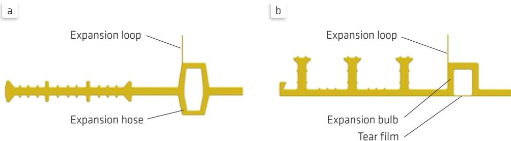
Fig. 5.94 Expansion bulb / hose (a) and tear flap closed expansion loop (b) on Sika PVC-P waterbars with their nail strap
