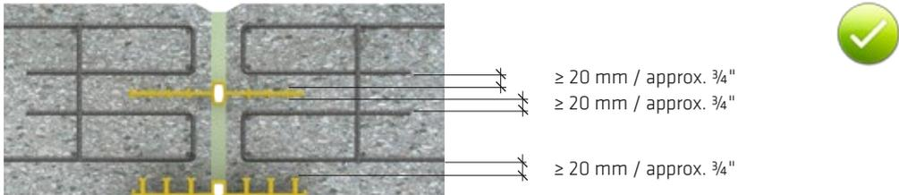
Fig. 5.25: Required minimum clearance between reinforcement and waterbar
