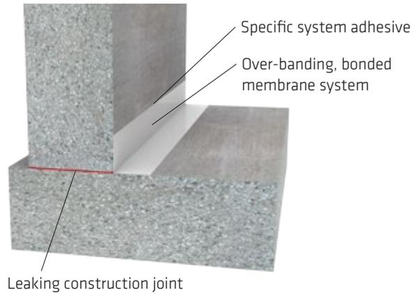
Fig. 15.6: Sealing of a construction joint with an over-banding membrane bonded to the concrete
