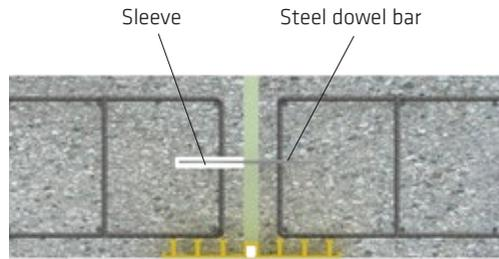
Fig. 5.33: Waterproofing of an expansion joint with transverse force transmission
