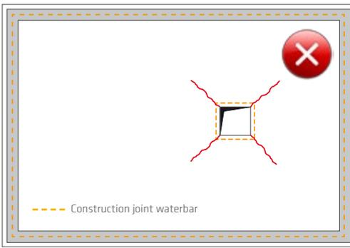
Fig. 2.6: Diagonal cracks at box-outs or shafts through a base slab
