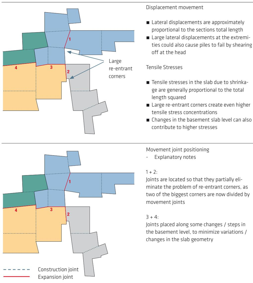
Fig. 3.2: Examples of suitable movement joint positioning
