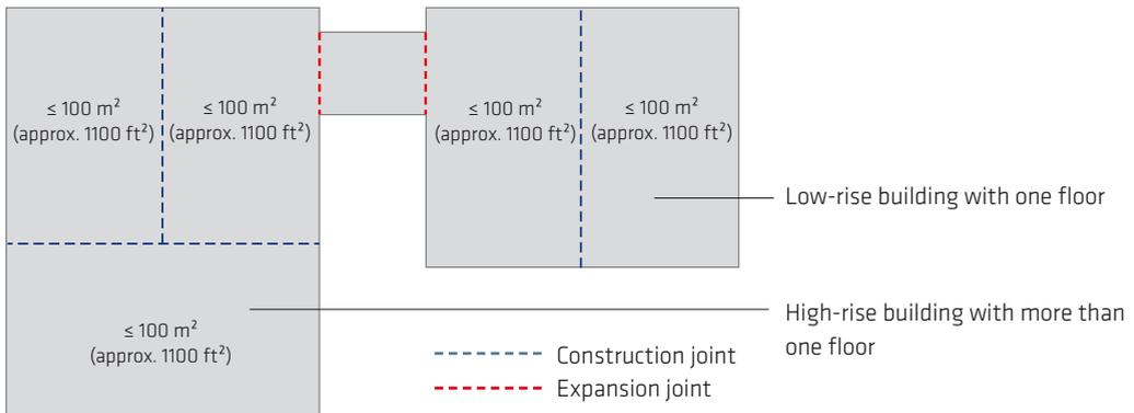
Fig. 2.5: Example of the typical layout for concrete construction and movement (expansion) joints
