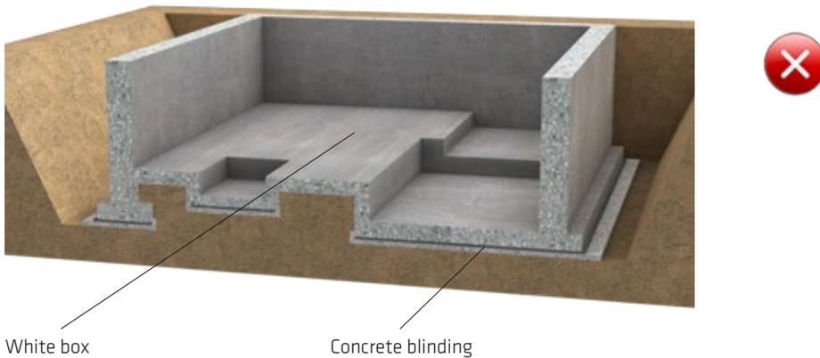
Fig. 2.14: Traditional design of reinforced concrete base slab, not suitable for the Sika White Box concept
