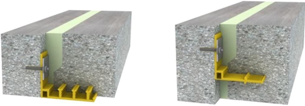
Fig. 5.15: External- and internal clamped waterstop, with one lec ( flange ) clamped to an existing structure
