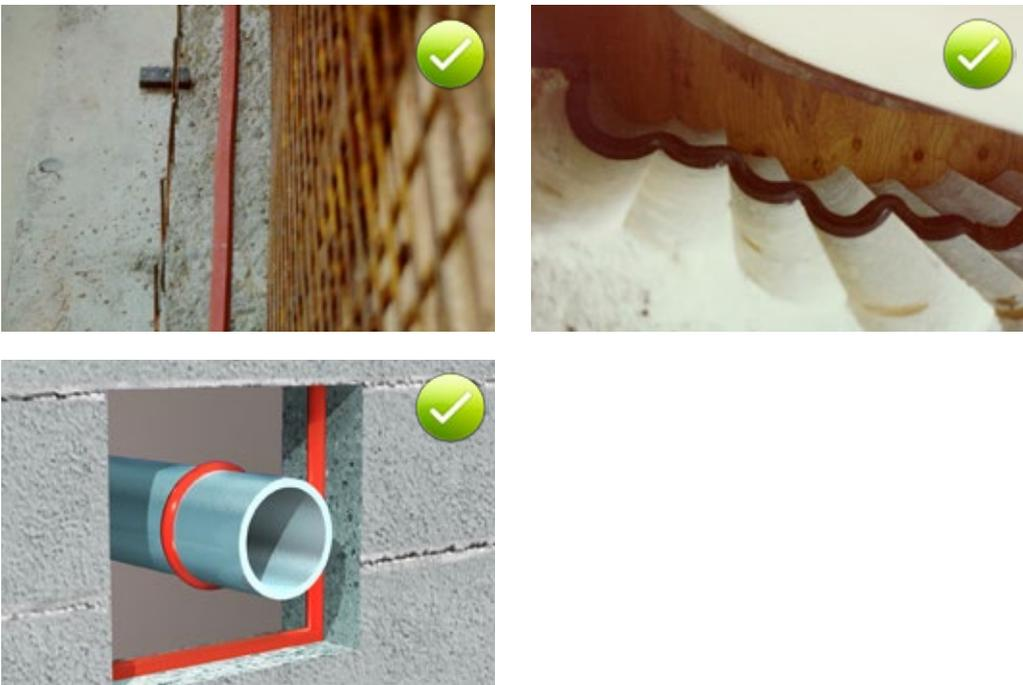
Fig. 8.1: Waterproofing with a swellable profile of: (a) a construction joint, (b) a connection joint with bored pile walls, (c) a pipe penetration
