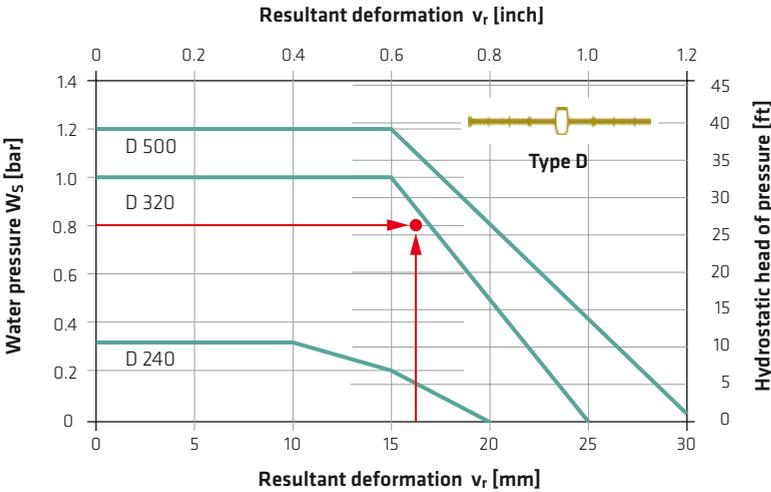
Fig. 5.46: Selection diagram for a Sika® Tricosal® Tricomer® internal expansion joint waterbar (example 1)
