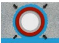
The injection tube is then clear and is available for further grouting at any time in the future. A leak test at defined water pressure is also possible at any time by injecting water.
