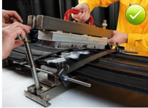
Fig. 5.87: Tensioning the vulcanizer
