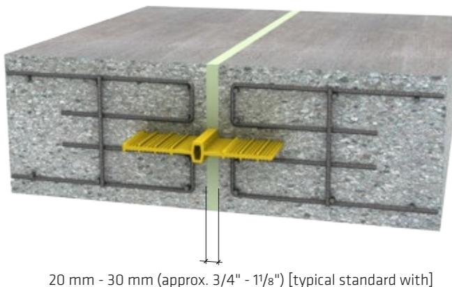
Fig. 3.1: Typically standard width for movement / expansion joints
