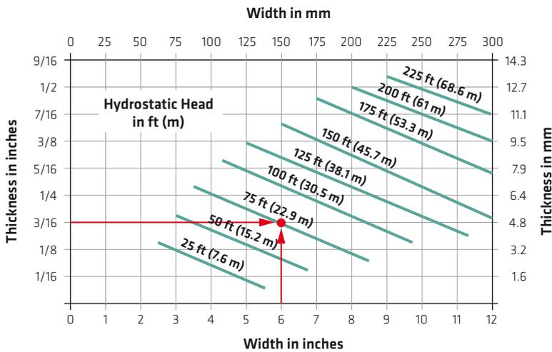
Fig. 5.40: Determination of the permissible water pressure (Hydrostatic Head) for an expansion joint waterbar (width: 6" / 152 mm, thickness: 3/16") from US Army Corps of Engineers "Waterstops and other joint materials" (EM1110-2-2102)
