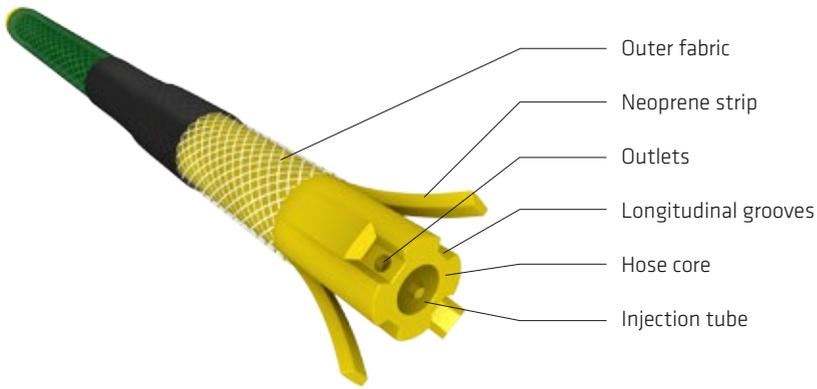
Fig. 9.6: Structure of the SikaFuko®VT injection hose
