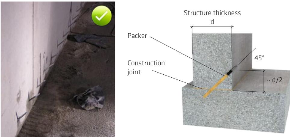
Fig. 15.5: Sealing of a horizontal construction joint by injection grouting through packers
