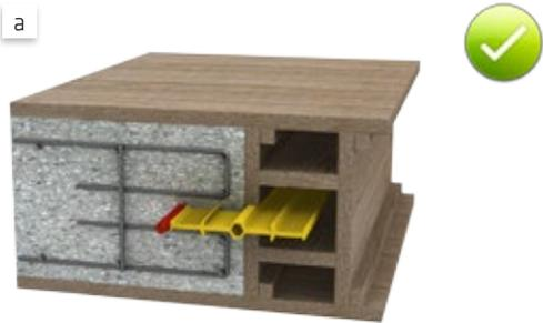
Fig. 5.101: Waterbar stop end formwork to the base slab
