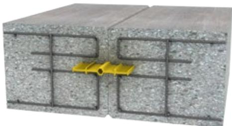
Waterproofing of a connection joint in the wall of a cut-and-cover tunnel with an expansion joint waterbar (if shear stress is ruled out)
