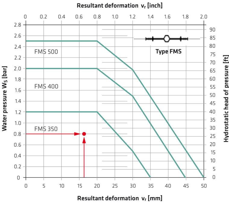
Fig. 5.55: Selection of a Sika® Tricosal® internal elastomeric expansion joint waterbar (type FMS)
