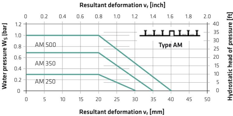
Fig. 5.53: Selection diagram for external elastomeric expansion joint waterbars (type: AM) according to DIN 18197 [7]
