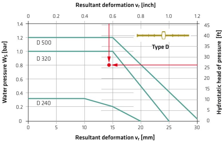
Fig. 5.48: Selection diagram for a Sika® Tricosal® Tricomer® internal expansion joint waterbar (example 2)
