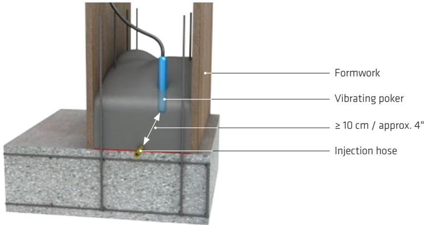
Fig. 9.17: Minimum clearances between injection hose and vibrating poker
