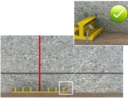
Fig. 5.99: Nailing external waterbars to the wall formwork through their nail strap section
