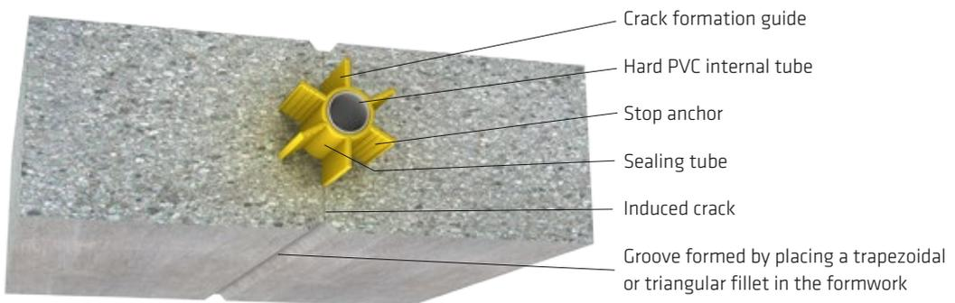
Fig. 11.2: Crack inducing sealing tube for forming and sealing induced crack wall sections (view onto the wall from above)
