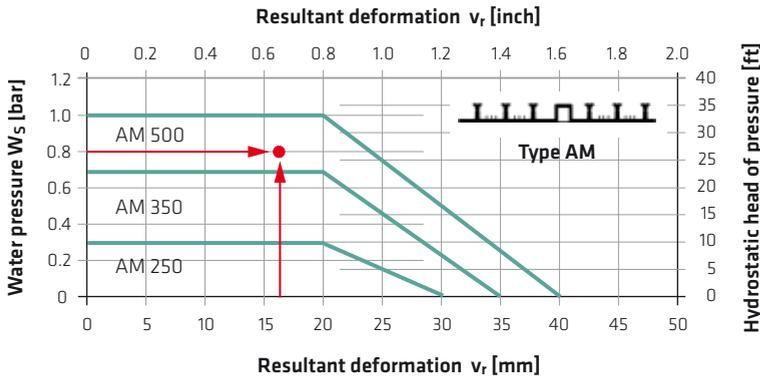
Fig. 5.56: Selection of a Sika® Tricosal® external elastomer expansion joint waterbar (type AM)
