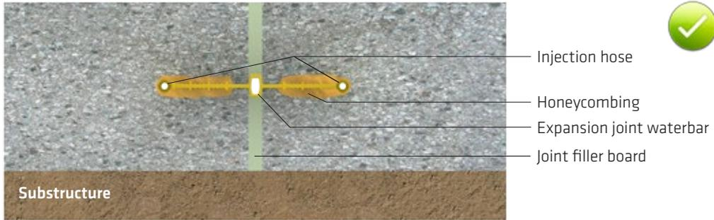
Fig. 15.9: Grouting of honeycombing and voids around the sealing part of the internal expansion joint waterbar through the installed injection hoses
