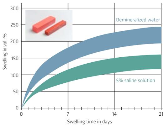
Fig. 8.5: Examples of the SikaSwell® A profiles swelling behaviour during free swelling in different solutions
