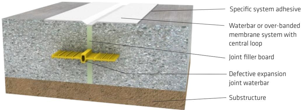
Fig. 15.13: Sealing of a leaking expansion joint with an over-banding membrane system
