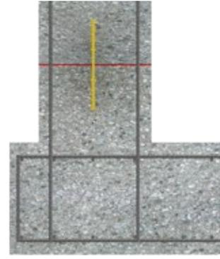
Fig. 5.20: Waterproofing of base slab-wall construction joint with an internal waterbar
