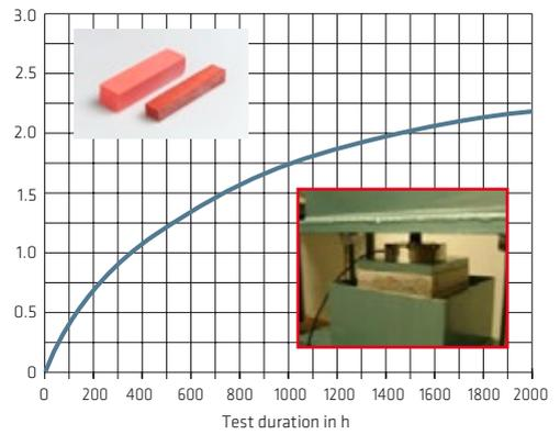
Fig. 8.6: Example of the swelling pressure development of cast-in SikaSwell® A profiles in distilled water [8]
