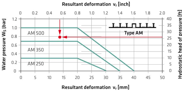
Fig. 5.59: Selection of a Tricosal® external elastomer expansion joint waterbar (type AM)
