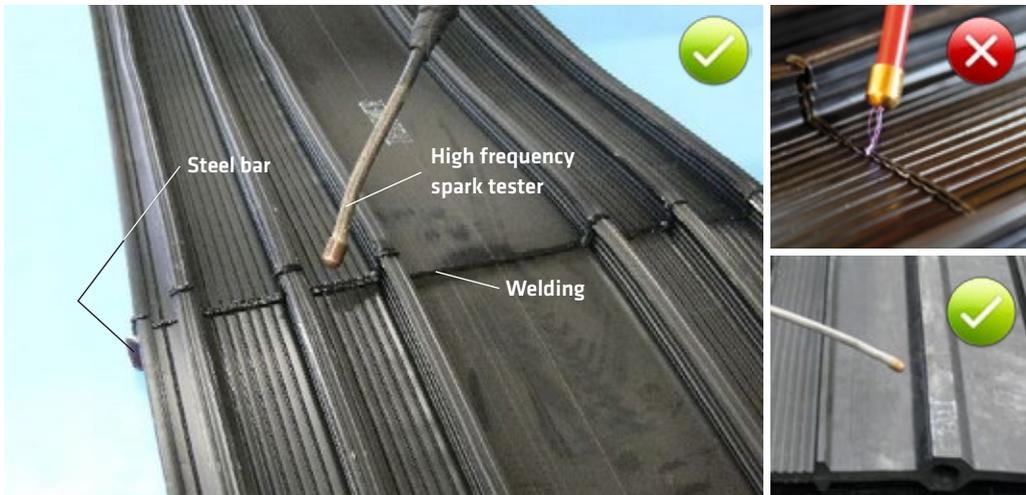
Fig. 5.85: Non-destructive testing of the impermeability of a weld with a high frequency spark tester; a visible spark passing through indicates a defect in the weld
