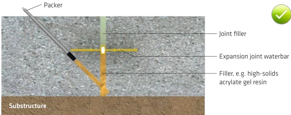
Fig. 15.10: Injection sealing of a joint with a damaged expansion part of the waterbar
