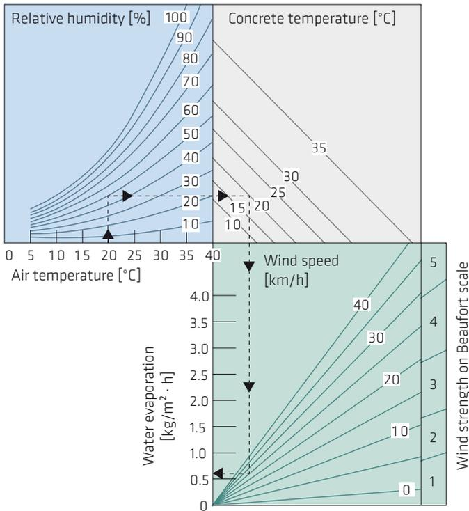
Fig. 2.25: Effect on water evaporation of relative air humidity and concrete temperature as well as wind speed (according to VDZ) [10]
