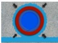
After injection, by applying a vacuum the injection tube is "sucked empty".
