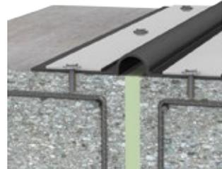
Fig. 5.14: Flanged waterbars with legs (flanges) clamped on both sides of the joint
