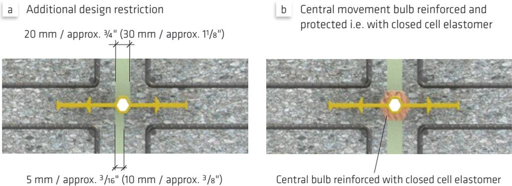
Fig. 5.31: Design of joints with anticipated compression load [8]
