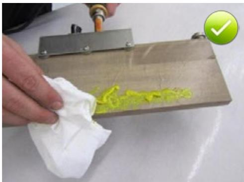
Fig. 5.70: Cleaning with a cloth to remove any welding residues from the welding blade before each welding operation
