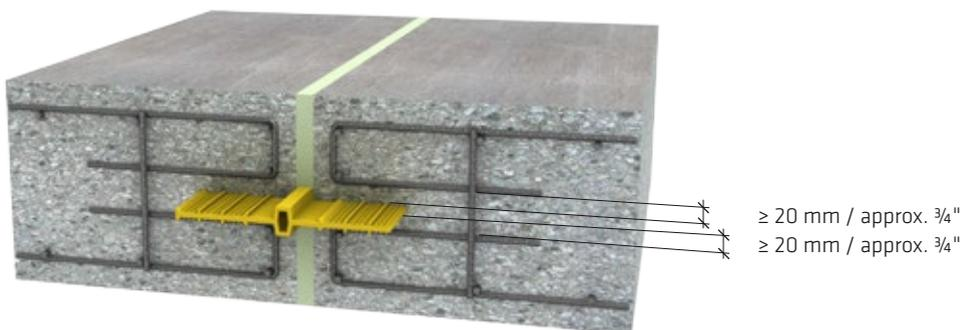
Fig. 3.6: Recommended minimum clearance between the reinforcement and joint waterbars
