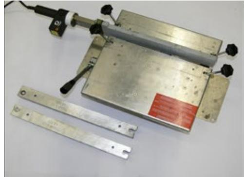
Fig. 5.72: SG 320 L automatic welding machine for the heat welding butt joints in thermoplastic waterbars
