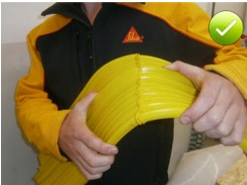
Fig. 5.82: Checking the joint strength by a simple cold bending test
