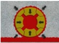
When pressure is removed, the neoprene strips seal the outlets and prevent backflow of the injection material.
