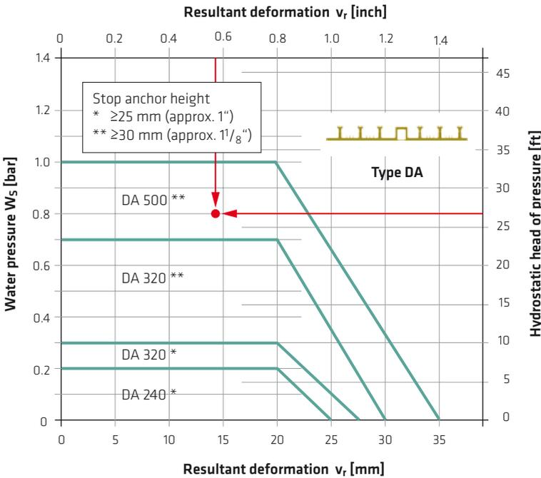
Fig. 5.47: Selection of a Sika® Tricosal® Tricomer® external construction joint waterbar (example 2)
