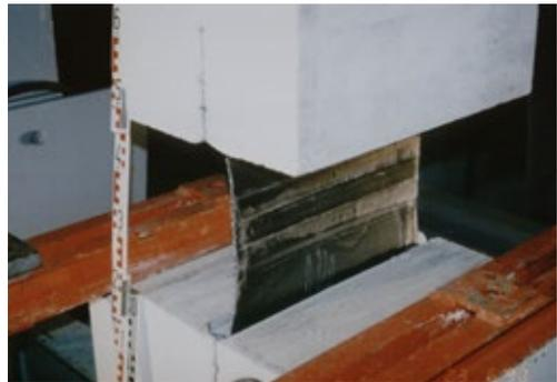
Fig. 5.49: Tensile test on a Sika® Tricosal® Tricomer® internal expansion joint waterbar 32 cm (approx. 12½") in width
