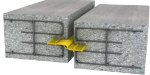
Fig. 5.12: Internal expansion joint waterbars - Method of operation
