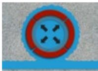
During injection grouting of the injection hose system, the neoprene strips are compressed outwards by the pressure from inside and so the injection material emerges into the construction joint.
