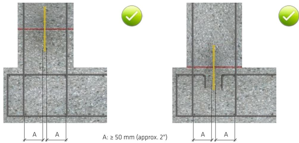
Fig. 5.27: Minimum clearance between an internal construction joint waterbar and the starter bars, using the example of a base slab-wall joint with a concrete kicker (left) and top reinforcement break (right)
