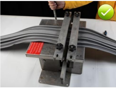
Fig. 5.75: Pressing the molten waterbar ends together with the closing lever mechanism again after lowering the blade
