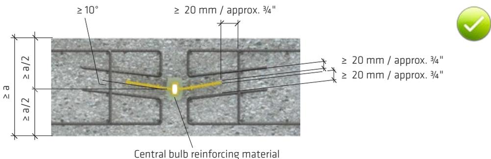
Fig. 5.32: Waterproofing of a connection joint in which shear strain occurs using an expansion joint waterbar with a reinforced central bulb (a = waterbar width)
