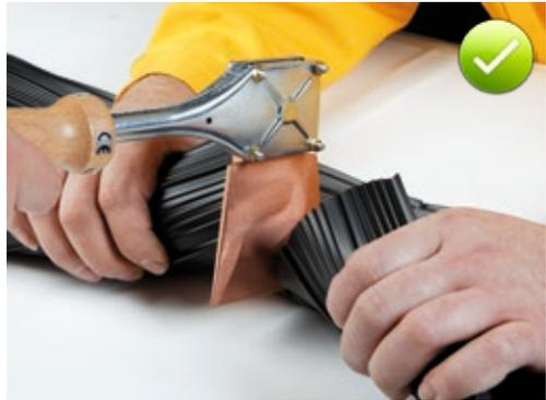
Fig. 5.78: Prefabrication of a butt joint with a welding axe
