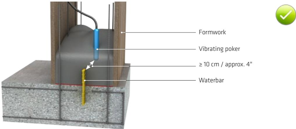
Fig. 5.104: Minimum clearance to the waterbar and other joint sealing parts of waterstop systems for compacting the concrete with a vibrating poker
