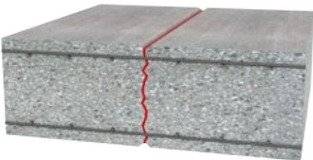
Controlled crack induced joints in walls for example, are intended for defined crack control by engineered concrete cross-section weakening and formation of a controlled point of cracking through the concrete. This relieves stresses due to temperature and shrinkage, which thereby prevents uncontrolled cracking in the wall. Cracking takes place in the designed and crack induced position instead.
