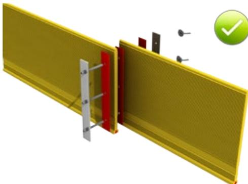
Fig. 7.9: Butt joint in a Sika® KAB 150 with clamping bars and swellable profile insert
