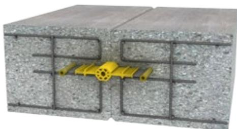
Waterproofing of a connection joint in the wall of a cut-and-cover tunnel with an elastomer waterbar with a reinforced central injection hose (if shear stress may occur)
