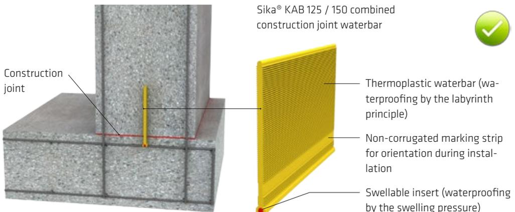
Fig. 7.1: Structure and installation positioning of Sika® KAB 125 / Sika® KAB 150
