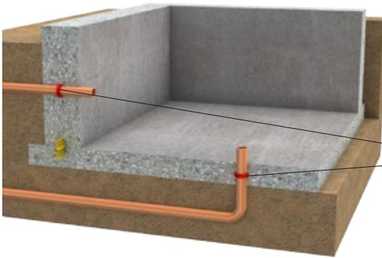
Waterproof sealing around pipe penetrations and conduits etc., e.g. sealing collars, swellable profiles or annular ring seal gaskets
