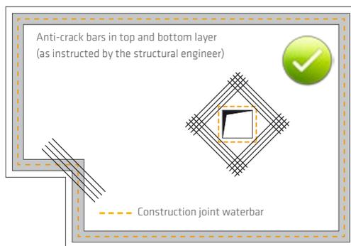
Fig. 2.18: Example of additional anti-crack bars at re-entrant corners, box-outs and other penetrations to prevent diagonal cracking
