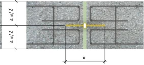
Fig. 5.19: Examples of correct waterbar configuration
