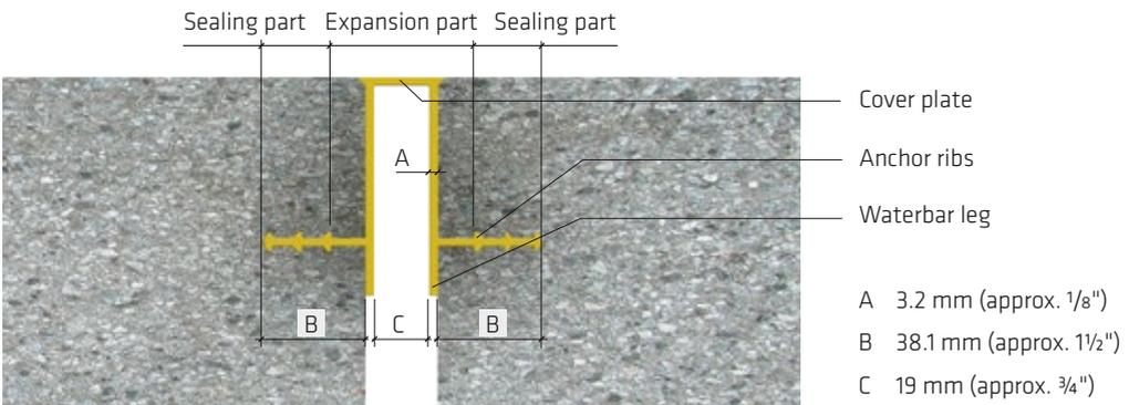
Fig. 14.3: Westec® end waterbar (type 631) complying with European Technical Approval ETA 04/0044 for LAU facilities [7]
