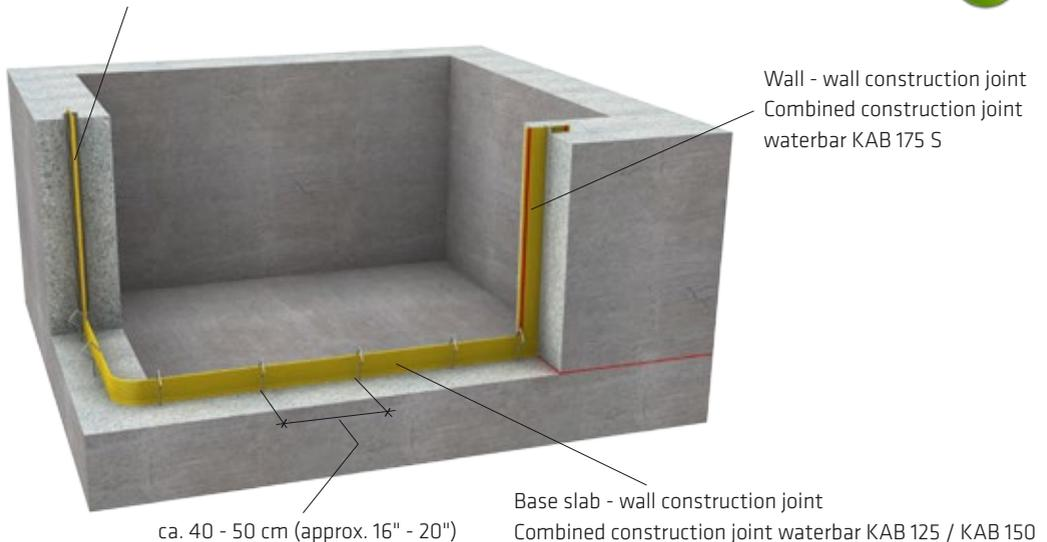
Fig. 7.3: Uses of Sika® KAB combined construction joint waterbars in construction joints and induced crack sections
