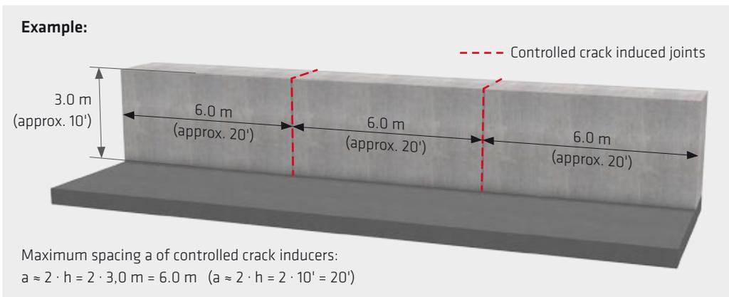
Fig. 3.4: Sample calculation for the spacing of controlled crack induced joints in a wall
