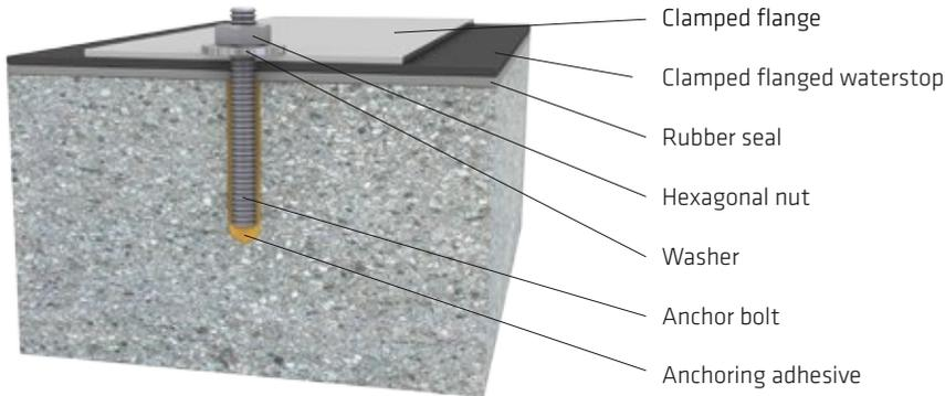
Fig. 13.3: Typical schematic layout of a clamped flange joint seal
