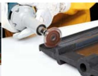
Grinding of the rubber surface
