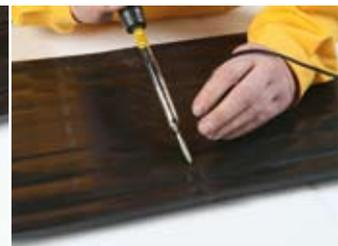
Strengthening with welding strip using welding tip
