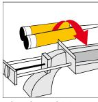
4. Place the cartridge into the application gun ready for use
