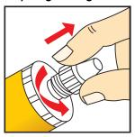
1. Unscrew and remove the cap
